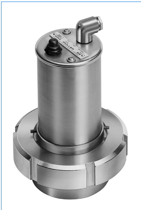
Sightglass light fitting type KLR 100 HD R80 K2, 100 W, 24 V, with built-in momentary push-button "D", mounted with flange collar "R 80" on screwed sightglass similar to DIN 11851, DN 80, PN 6.
