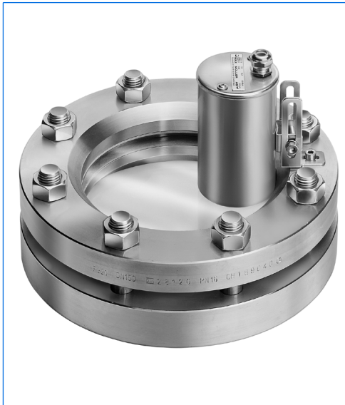
Sightglass light fitting type KLR PowerLED Sch, 7 W, 230–240 V, mounted with tilting hinge "Sch" on sightglass to DIN 28120, DN 150, PN 10, for application "view and light through one assembly".
