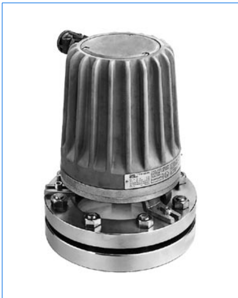
High performance sightglass light fitting type 100 deHN, 100 W, 24 V, Ex d e IIC T4 Gb, Ex t IIIC T130°C Db IP67, Ex II 2 G + D, foot ring fixation on sightglass to DN 28120, PN 10, DN 125
