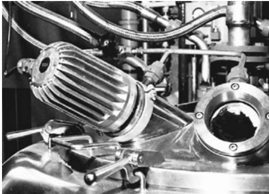
CHEMLUX® sightglass light fitting, type L 20 dH Sch, 20 W, 230 V, Ex d e IIC T5 Gb, Ex t IIIC T95°C Db IP67, Ex II 2 G + D, with fixation "Sch" on a basket centrifuge
