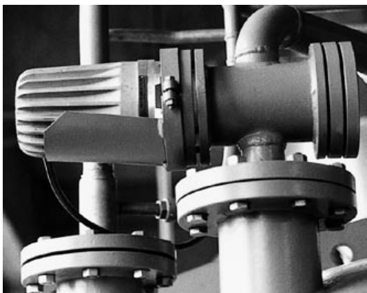
CHEMLUX® sightglass light fitting, type L 20 deH M sp, 20 W, 24 V, Ex d e IIC T5 Gb, Ex t IIIC T95°C Db IP67, Ex II 2 G + D, mounted with an opal glass screen "M" on a pipeline flow indicator
