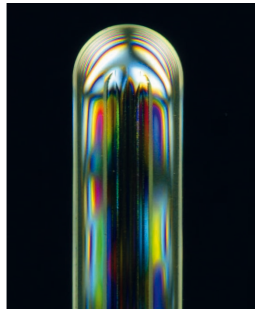
Special tempered MAXOS® glass under polarized light.
