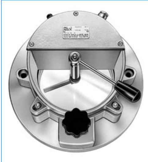
Hinged illuminated sightglass type KSGB 125. Terminal voltage of built-on light fitting 24 V, nominal rating 50 or 100 watts. Built-in wiper, series W.
