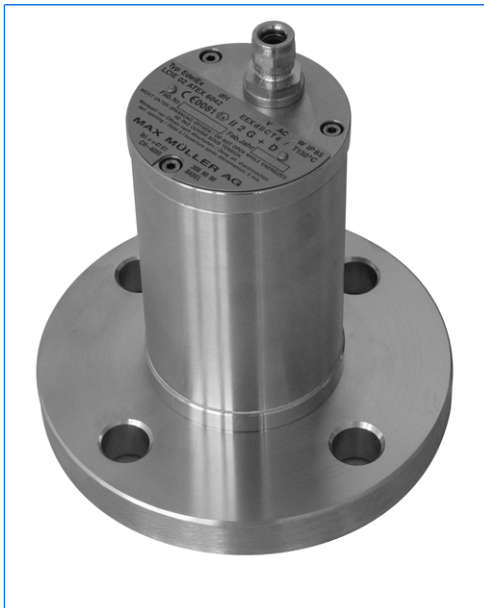
Sightglass light fitting type EdelEx STERI-LINE 20 dH, 24 V, 20 W, Ex d IIC T4 Gb, Ex t IIIC T130°C Db IP67, Ex II 2 G + D, on metal fused sightglass flange
