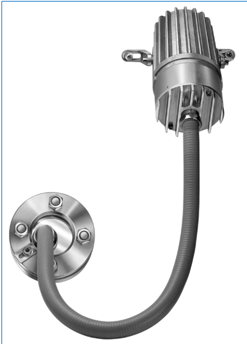
Fibre-optic lightpipe light fitting for use in hazardous areas with built-in timer "V", type fibroLUX® 5035 X1 W2 V, Ex de IIC T4 Gb, Ext IIIC T130°C Db IP67, Ex II 2 G + D, 35 W, 230 V, fixation of the light source by fixation legs "X1", fixation of the lightpipe by universal support "W2" onto sightglass to DIN 28120, DN 40, PN 10
