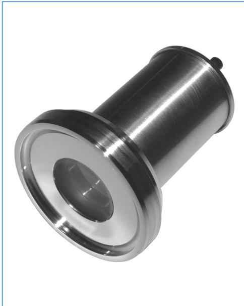
Light fitting miniLUX STERI-LINE, type BKVLR DA LED, ca. 2 W, 24 V, mounted on metal fused sightglass to DIN 11864-1
