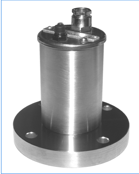
Sightglass light fitting type BKVLR 20 HDA, 20 W, 24 V, with built-in momentary push-button "D", on metal fused sightglass for aseptic flange connections to DIN 11864-2, DN 50
