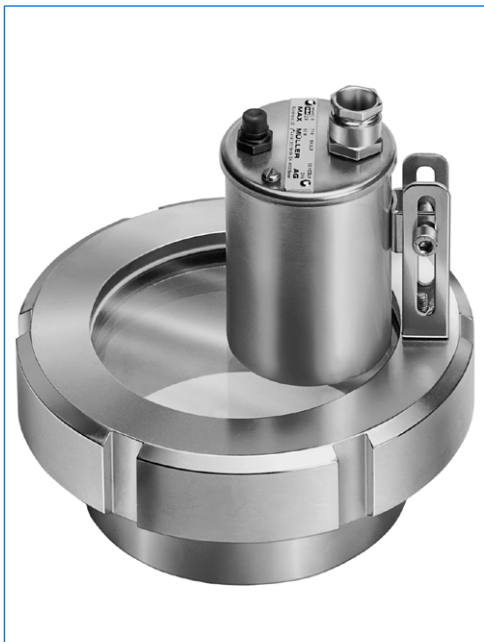
Sightglass light fitting type BKVLR 50 HDSch1, 50 W, 24 V, with built-in momentary push-button "D", mounted with tilting hinge "Sch1" on sightglass similar to DIN 11581, DN 100, PN 6, for application "view and light through one assembly".
