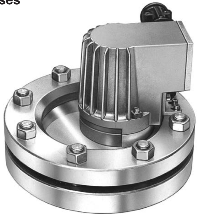
Type KEL 20 deH W, Ex d e IIC T4 Gb, Ex t IIIC T130°C Db IP67, Ex II 2 G + D, 230 V, 20 W, mounted on circular sightglass to DIN 28120, DN 125, PN 10, in 1 port version.
